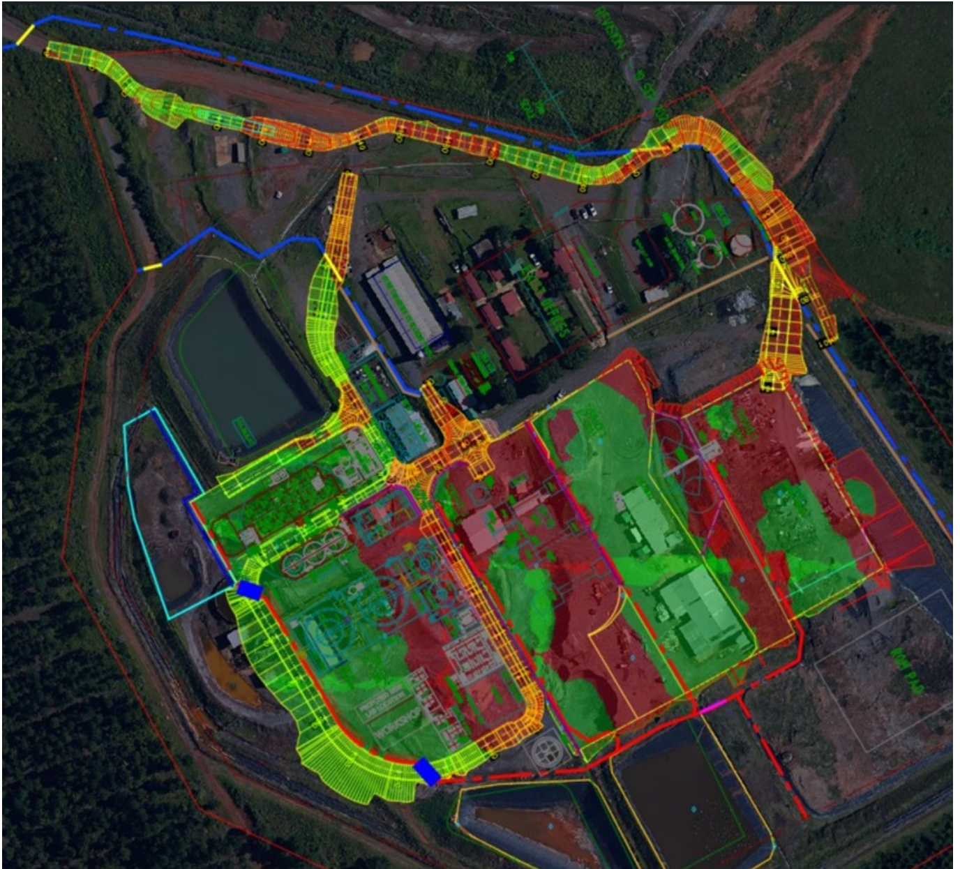
Figure 6: Bulk Earthworks cut and fill requirements (Red area to be cut and Green to be filled)
