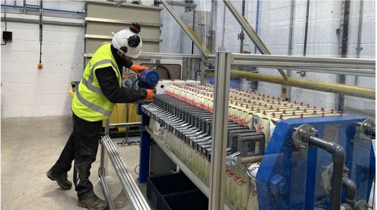
Figure 5: Operator preparing Filter Press for mixed REO cake production.
