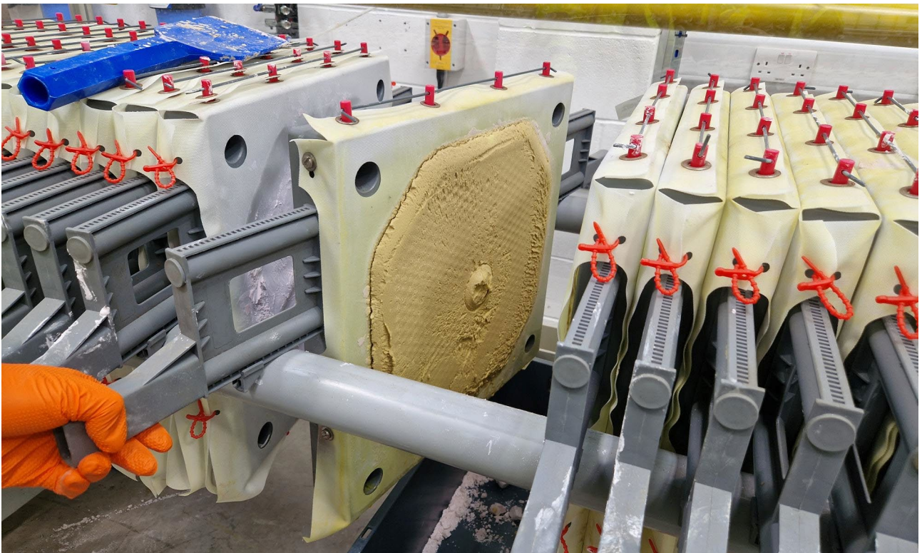
Figure 6: Cake intermediate product prior to removal from filter press cloths.
