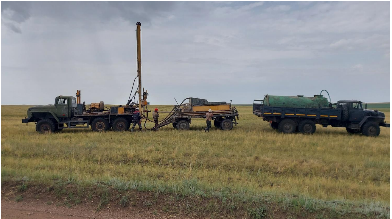
Figure 1 - Water Core Drilling Rig at Kenesar.
