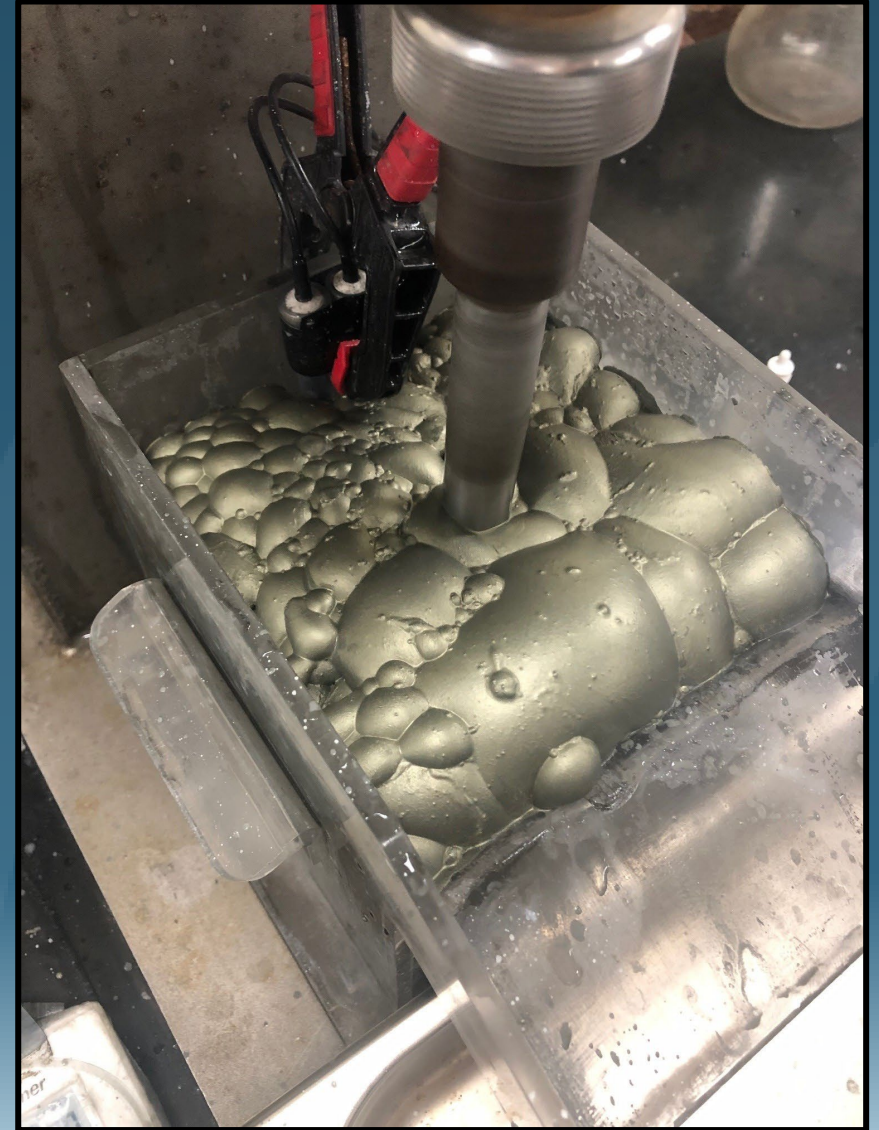
Sulphide flotation of Callisto sample from NRCD337
