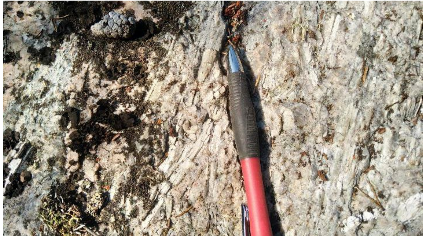
Spodumene (identifiable as cleaved, elongate white mineral) in pegmatite outcrop from sample location BHDS-23, Big Hill Project area. This area was channel sampled in the field study (at location BHDS-23-C01) and contained up to 2.6% Li 2 O over a metre 3
