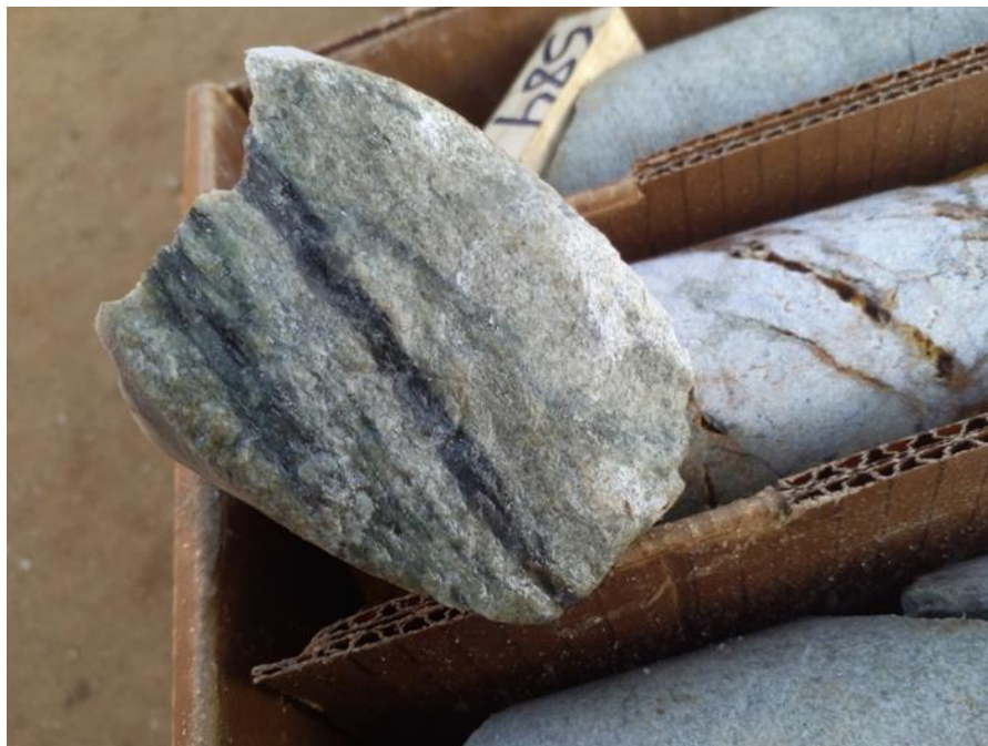
GDD02 - Quartz-sericite-pyrite altered intrusive with quartz-sulphide veins.
