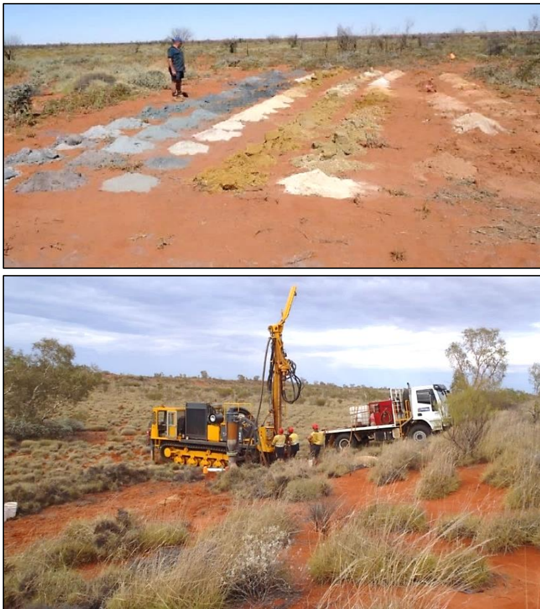
Figure 6.14: RC drilling at the Webb tenements – a total of 83 drillholes have been completed, with drillhole spoils (top image) being analysed for KIM and diamond content
