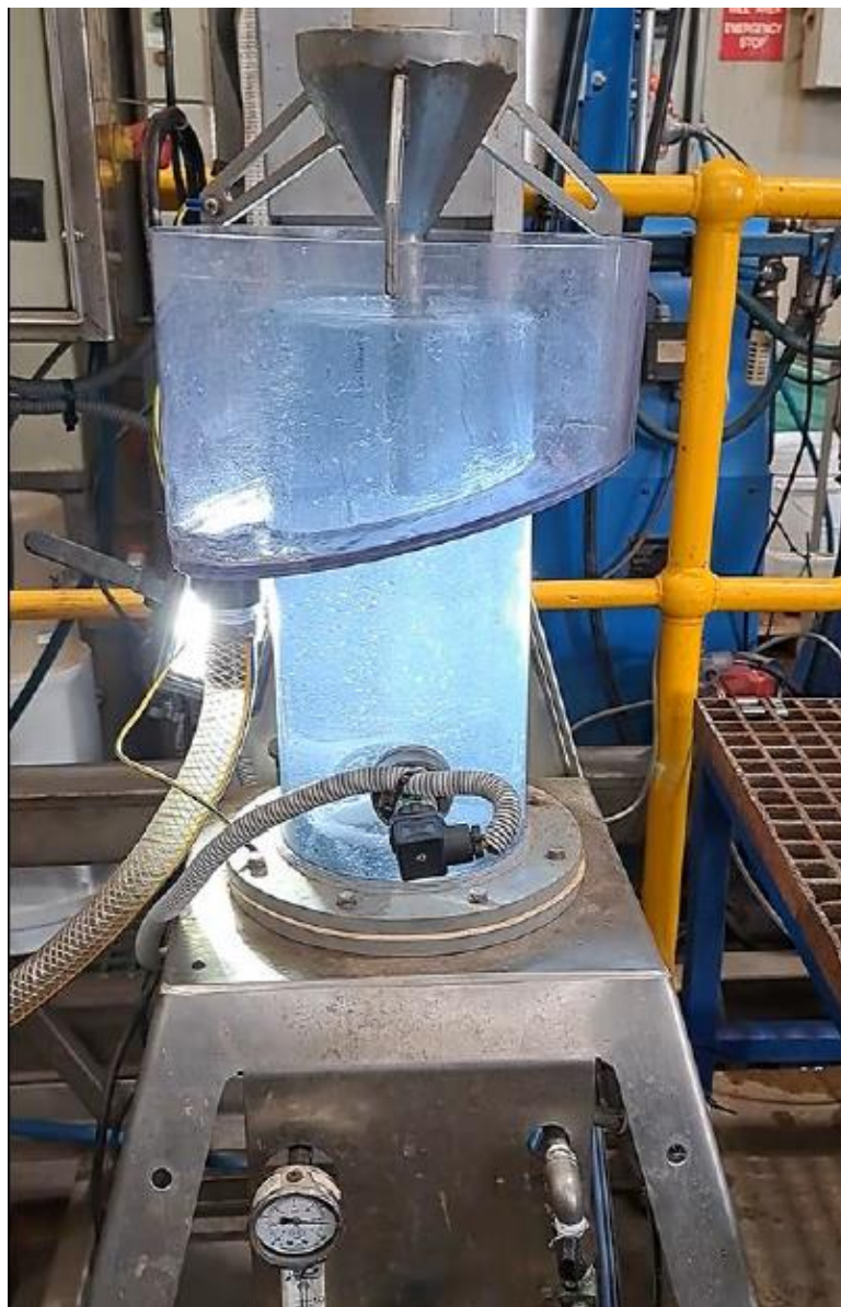
Figure 1: Eriez 6" Laboratory HydroFloat Setup
