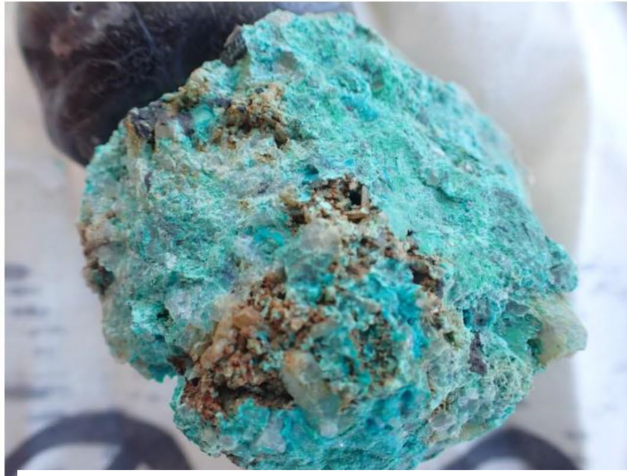
Sample ESS02045 - A white, frosty to glassy quartz vein hosting abundant drusy cavities lined with euhedral prismatic quartz crystals encrusted with supergene malachite and chrysocolla developed over sooty tenorite (Coordinates Location 774873E 8007987N)
