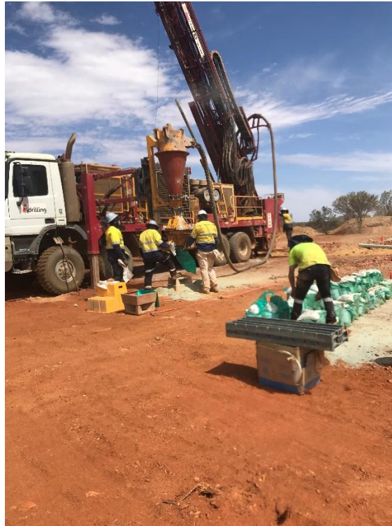
Figure 2: RC drill rig in operation, sampler in foreground sieving samples for geological logging
