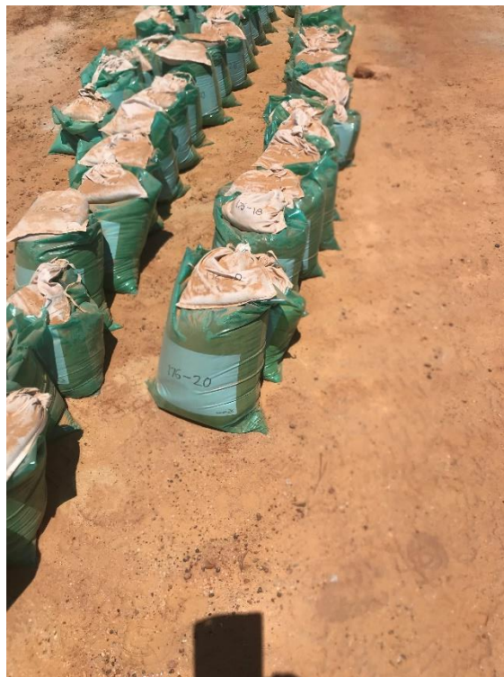
Figure 4: 1m sample from drill rig (green bag) ; 1m sample splits for possible lab submission (calico white bag)
