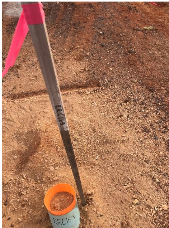
Figure 8: Labelled peg showing drilled hole location and capped collar
