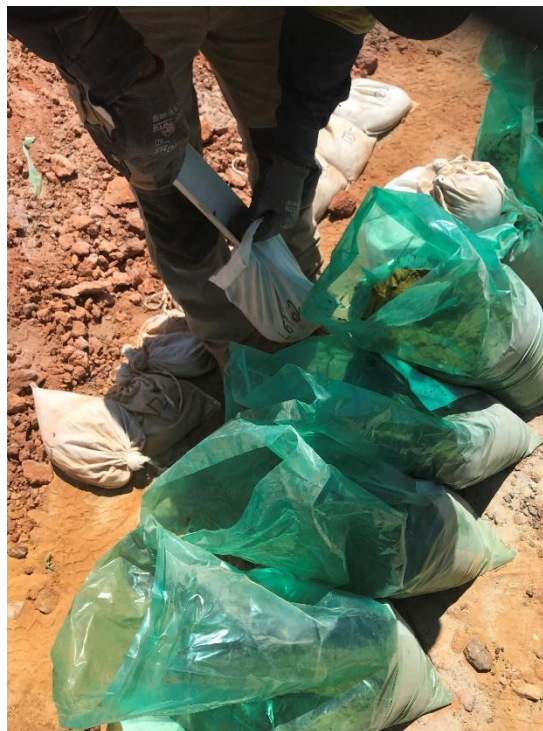
Figure 6: Compositing 1m samples into 2m to 4m composites using the spear method
