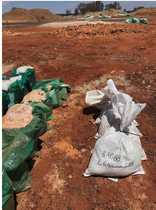
Figure 7: Polyweave bags showing samples selected for assay ; polyweave bags then placed in Bulka Bags for transport to laboratory
