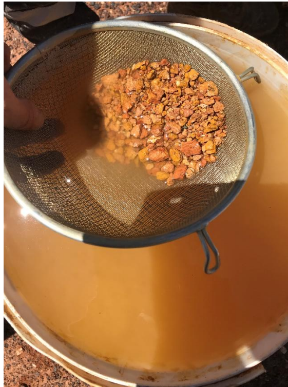
Figure 3: Sieving sample to prepare chips for geological logging
