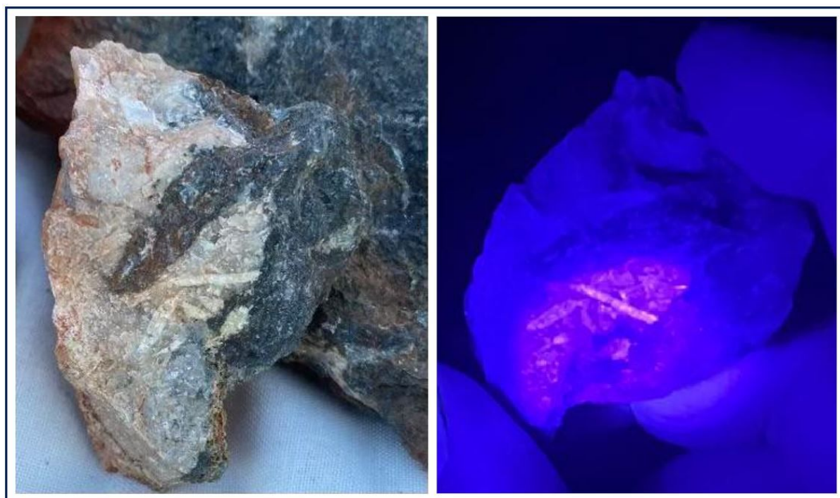
Figure 4. – Hand-specimen of spodumene crystals in LCT pegmatite showing strong pink fluorescence, a characteristic feature under long-wavelength UV light. See location of sample in Figure 5.
