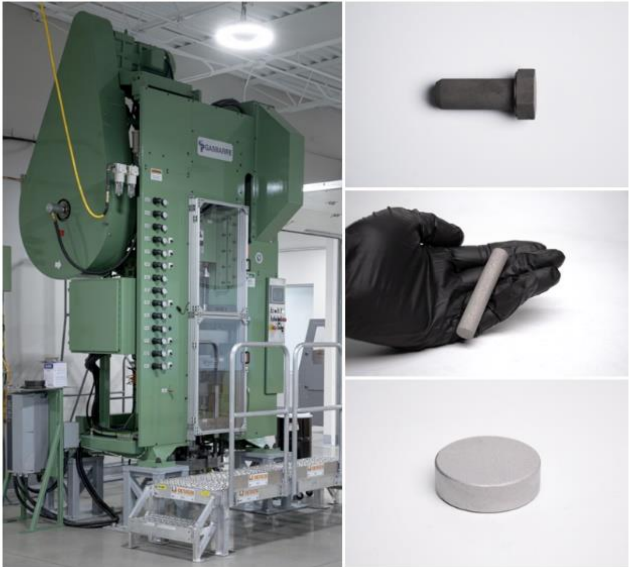
Figure 4: Powder metallurgy machinery at the AMC and production of consolidated titanium components
