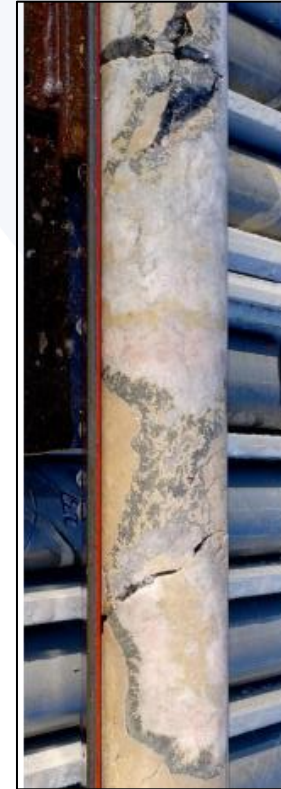
Drill core from BPD09 (about 223.5m down-hole depth) showing siderite (cream) and barite (white) veining. Abundant grey tetrahedrite is rimming colloform siderite-barite veining. Assay result: 4m @ 0.53% Cu, 10 g/t Ag, 0.21% Sb from 223 m
