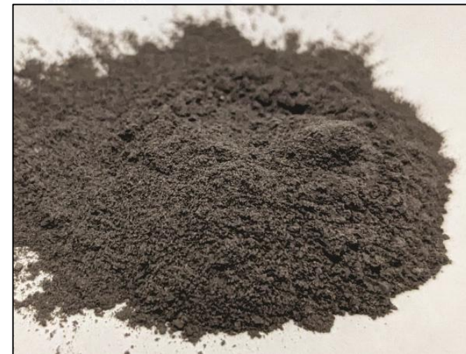
Below: 37% Sb (antimony sulphide) precipitated from leach liquor
