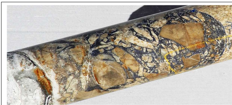
Fig 10. Core oriented frame photos of full HQ core for hole 23CAEDD021 at 142.6m (LHS) and 148.16m (RHS) . Hole oriented -steeply to south west : drilling inclined -70 degrees to 230° mag. View looking south east. Sheeted quartz-pyrite-chlorite-actinolite? veins with 1cm bleached sericite selvages. Cutting crowded plagioclase , biotite phyric porphyritic diorite. Veins display typical porphyry style affinities eg B-veins or D veins?. LHS veins dipping 85° to north north east (025° mag). RHS veins dipping 80° to NNE (025° mag)
