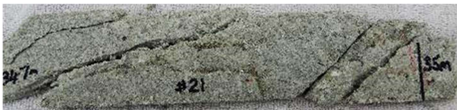
Intensely sericite and argillic altered crowded diorite porphyry with strong disseminated pyrite development , cut by clay rich veins & shears : CAE Hole 21, 23.1m . Note .1m interval 23m-24m : 5.19 g/t Au, 0.1% Cu, 23 g/t Ag, 10.62% S.
