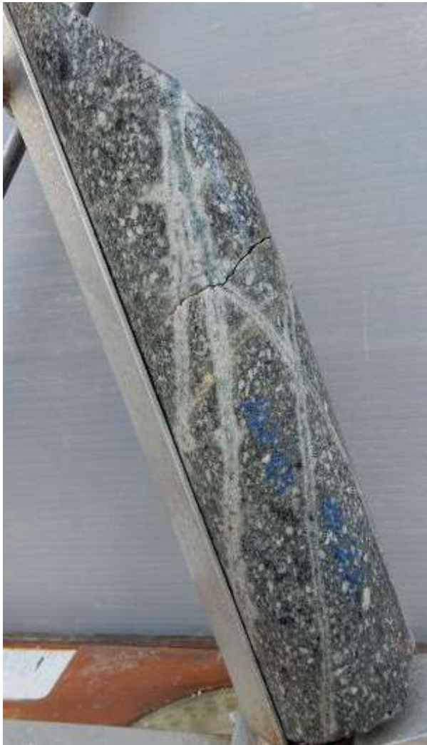
Fig 10. Core oriented frame photos of full HQ core for hole 23CAEDD021 at 142.6m (LHS) and 148.16m (RHS) . Hole oriented -steeply to south west : drilling inclined -70 degrees to 230° mag. View looking south east. Sheeted quartz-pyrite-chlorite-actinolite? veins with 1cm bleached sericite selvages. Cutting crowded plagioclase , biotite phyric porphyritic diorite. Veins display typical porphyry style affinities eg B-veins or D veins?. LHS veins dipping 85° to north north east (025° mag). RHS veins dipping 80° to NNE (025° mag)
