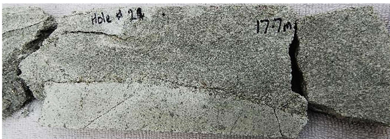
Fig 5. Photo half HQ core : intensely sericite and argillic altered porphyry and diorite dyke with strong disseminated pyrite development . CAE Hole 21 at 17.7m . Note 1m interval 17m-18m : 1.17 g/t Au, 0.06% Cu, 8.1 g/t Ag, 4.24% S.
