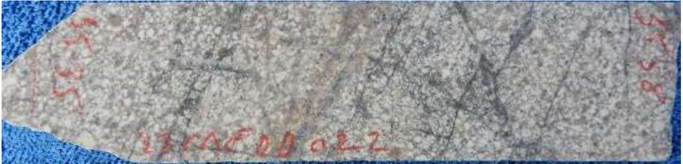
Fig 14. Sericite altered crowded diorite porphyry veins of quartz-pyrite with orange K feldspar? Selvedges, minor irregular stockwork of hairline pyrite. CAE Hole 22, 55.35m .
