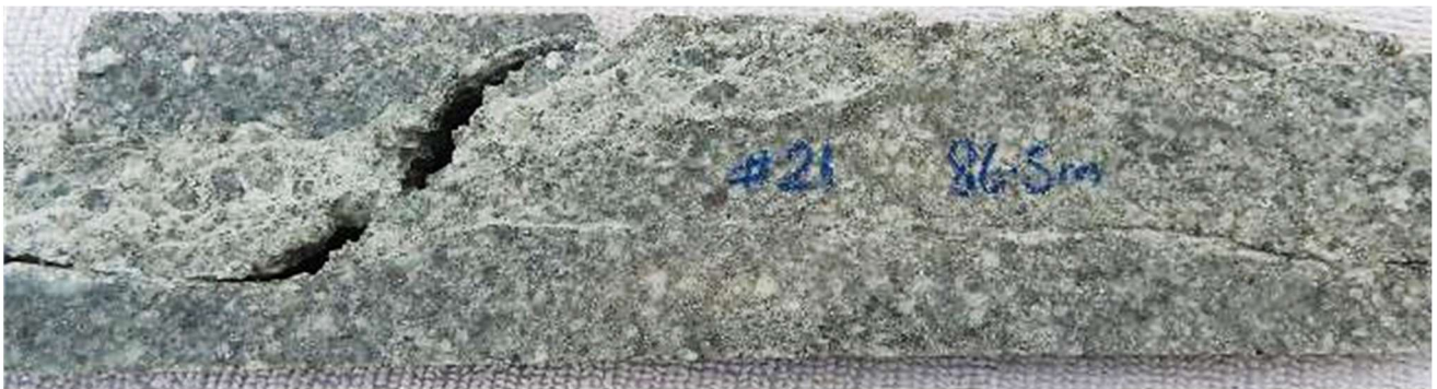
Fig 7. Intensely sericite and argillic altered crowded diorite porphyry with strong disseminated pyrite development: CAE Hole 21, 86.5m . Note .1m interval 86m-87m : 2.42 g/t Au, 0.02% Cu,12.3 g/t Ag, 3.70% S.
