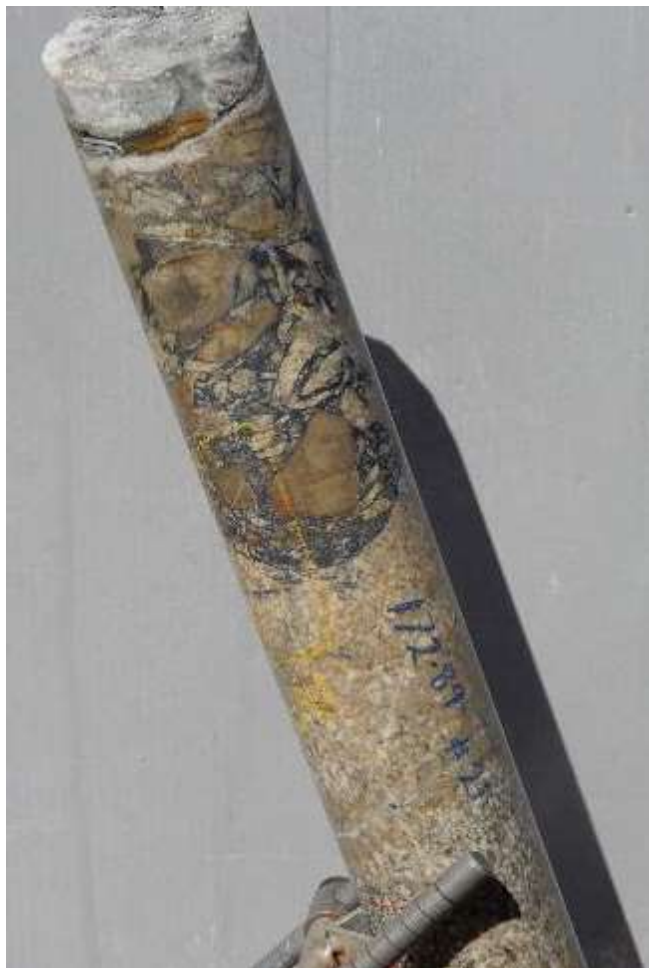
Fig 13 RHS. Core oriented frame photos of full HQ core for hole 23CAEDD022 at 76.6m . Hole oriented -steeply to north east : drilling inclined -75 degrees to 046° mag. View looking south west. Sulphidic argillized matrix supported breccia zone with angular clasts bleached hornfels and clay altered diorite porphyry . Breccia zone dipping shallowly -25° to south east (130° mag), striking 040°.
