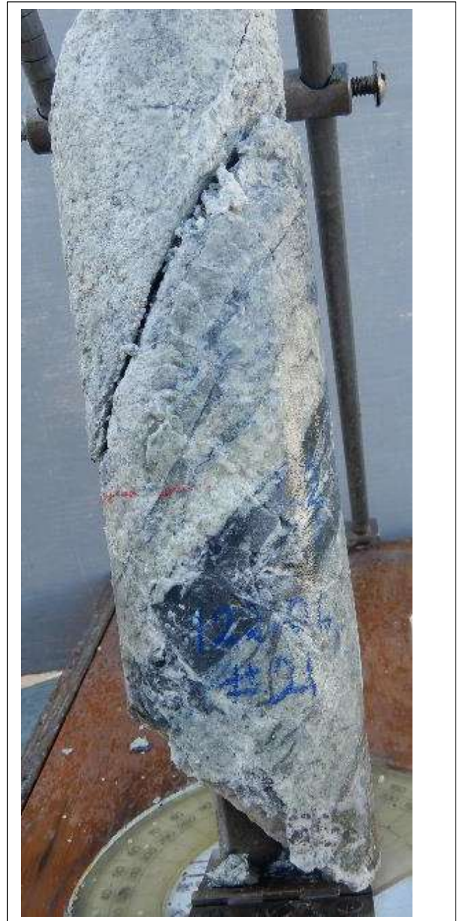
Fig 9. Core oriented frame photos of full HQ core for hole 23CAEDD021 at 110.25m (LHS) and 122.6m (RHS) . Hole oriented -steeply to south-west: drilling inclined -70 degrees to 230 degrees magnetic. View looking north-east.
