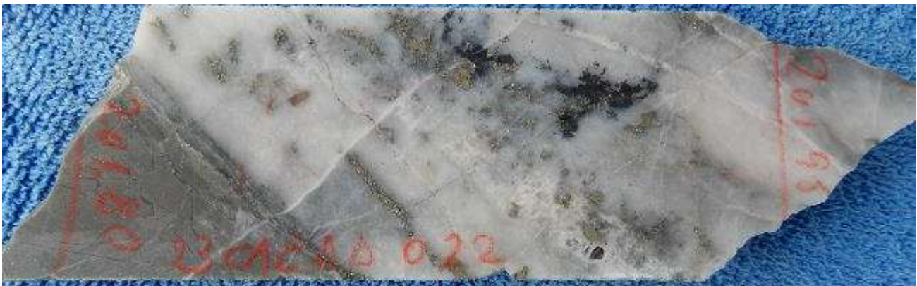
Fig 15 Quartz pyrite , galena, black sphalerite vein cutting sericite altered hornfels.CAE Hole 22, 201.9m . Interval 201m – 204m : 3m @ 2.45 g/t Au, 0.09% Cu,13.1 g/t Ag, 2.64% S, 0.3% Pb,0.18% Zn.
