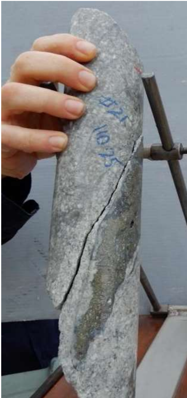
Fig 9. Core oriented frame photos of full HQ core for hole 23CAEDD021 at 110.25m (LHS) and 122.6m (RHS) . Hole oriented -steeply to south-west: drilling inclined -70 degrees to 230 degrees magnetic. View looking north-east.
