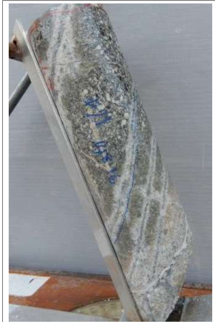
Fig 10. Core oriented frame photos of full HQ core for hole 23CAEDD021 at 142.6m (LHS) and 148.16m (RHS) . Hole oriented -steeply to south west : drilling inclined -70 degrees to 230° mag. View looking south east. Sheeted quartz-pyrite-chlorite-actinolite? veins with 1cm bleached sericite selvages. Cutting crowded plagioclase , biotite phyric porphyritic diorite. Veins display typical porphyry style affinities eg B-veins or D veins?. LHS veins dipping 85° to north north east (025° mag). RHS veins dipping 80° to NNE (025° mag)
