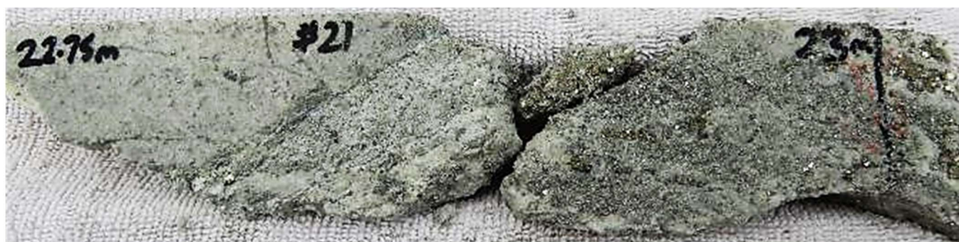
Fig 4. Photo half HQ core : intensely sericite and argillic altered crowded diorite porphyry with strong disseminated pyrite development , cut by pyrite veins : CAE Hole 21 at 23m . Note 1m interval 22m-23m : 1.07 g/t Au, 0.06% Cu, 3.8 g/t Ag, 2.81% S.
