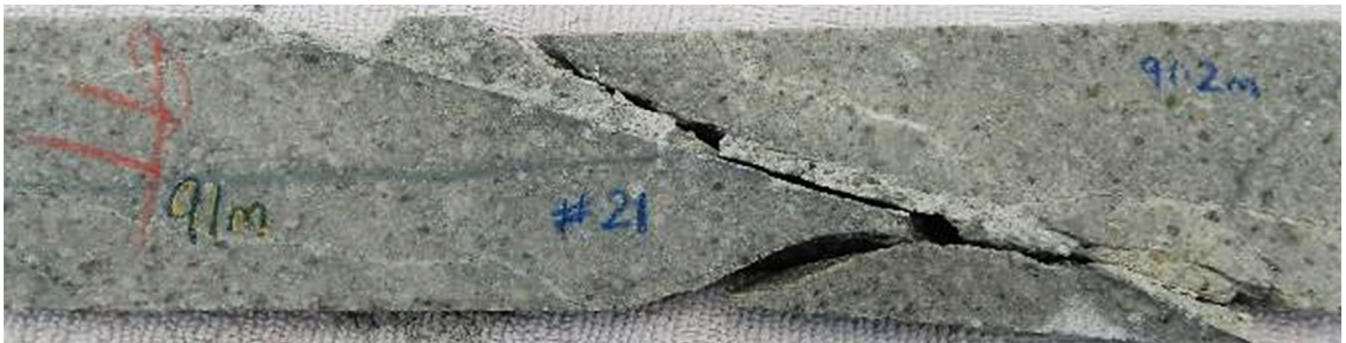
Fig 8. Intensely sericite and argillic altered crowded diorite porphyry with quartz pyrite clay fracture fillings and veins, disseminated pyrite : CAE Hole 21, 91m . Note .1m interval 91m-92m : 3.32 g/t Au, 0.09% Cu,10.2 g/t Ag, 2.53% S.
