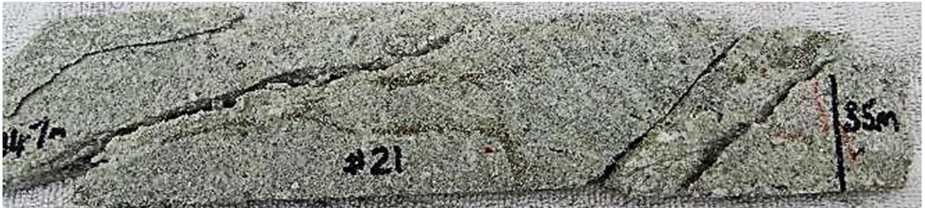
Fig 6. Intensely sericite and argillic altered crowded diorite porphyry with strong disseminated pyrite development , cut by pyrite veins : CAE Hole 21, 34.7m . Note .1m interval 34m-35m : 6.21 g/t Au, 0.02% Cu,9.1 g/t Ag, 8.41% S.
