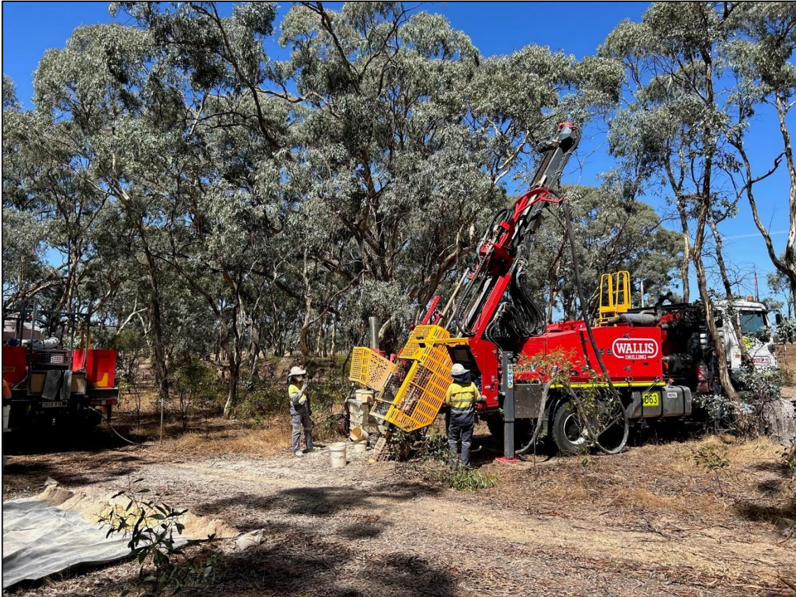
AC Drilling in Crown Land
