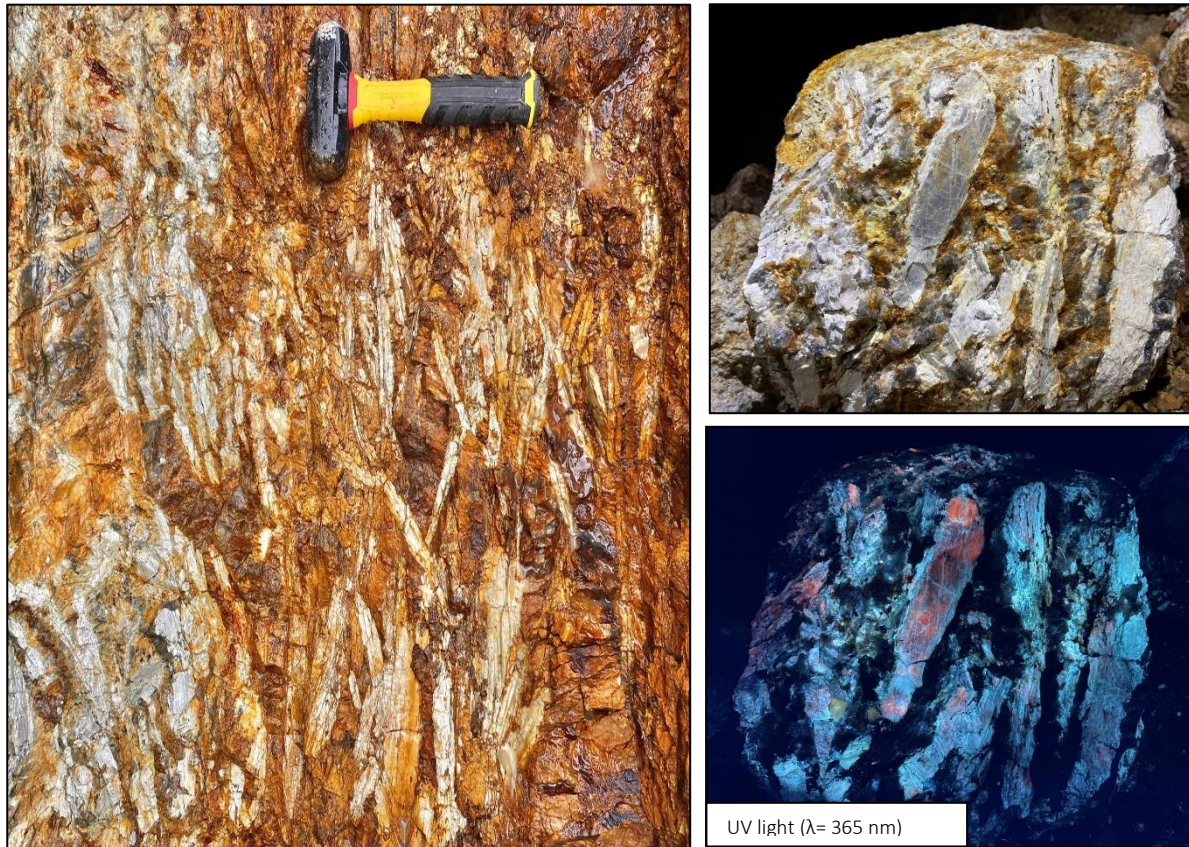
Figure 3: Spodumene concentrated in the walls and floor of Trench 1, elongate minerals are lithium spodumene. UV highlighting fluorescent spodumene crystals within weathered pegmatite at Trench 1.
