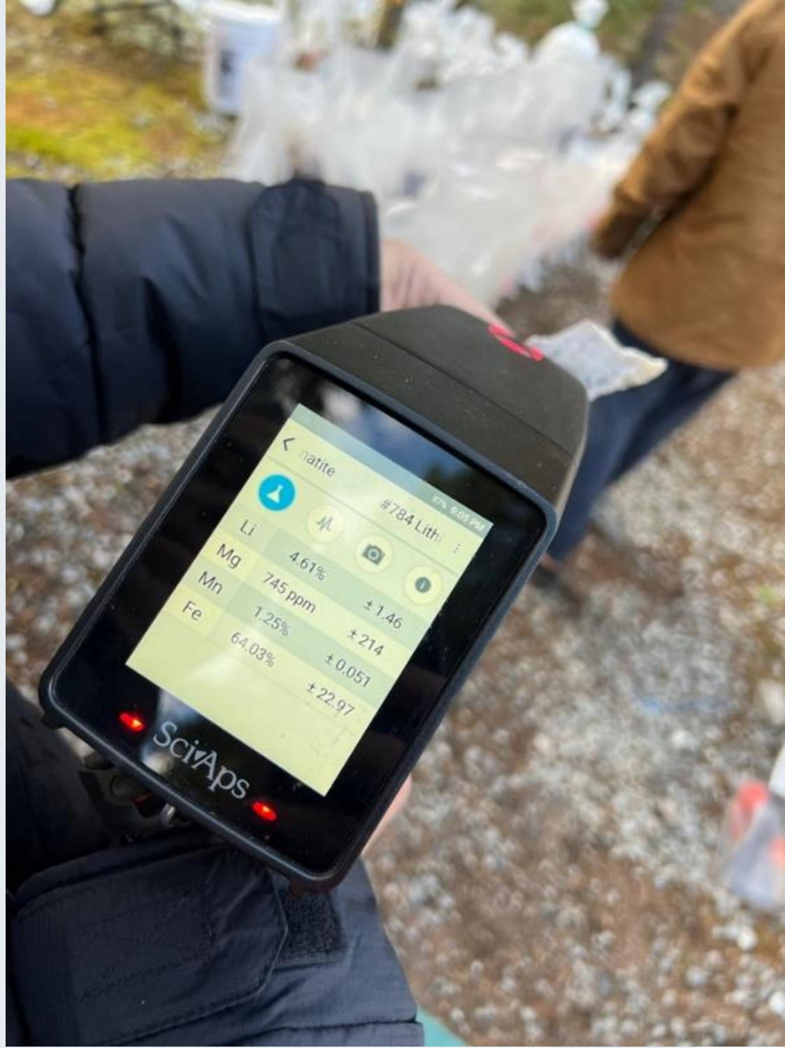
Figure 3 - Fresh rock channel sample from Warhawk with lithium mineralisation indicated by LIBS. 2
