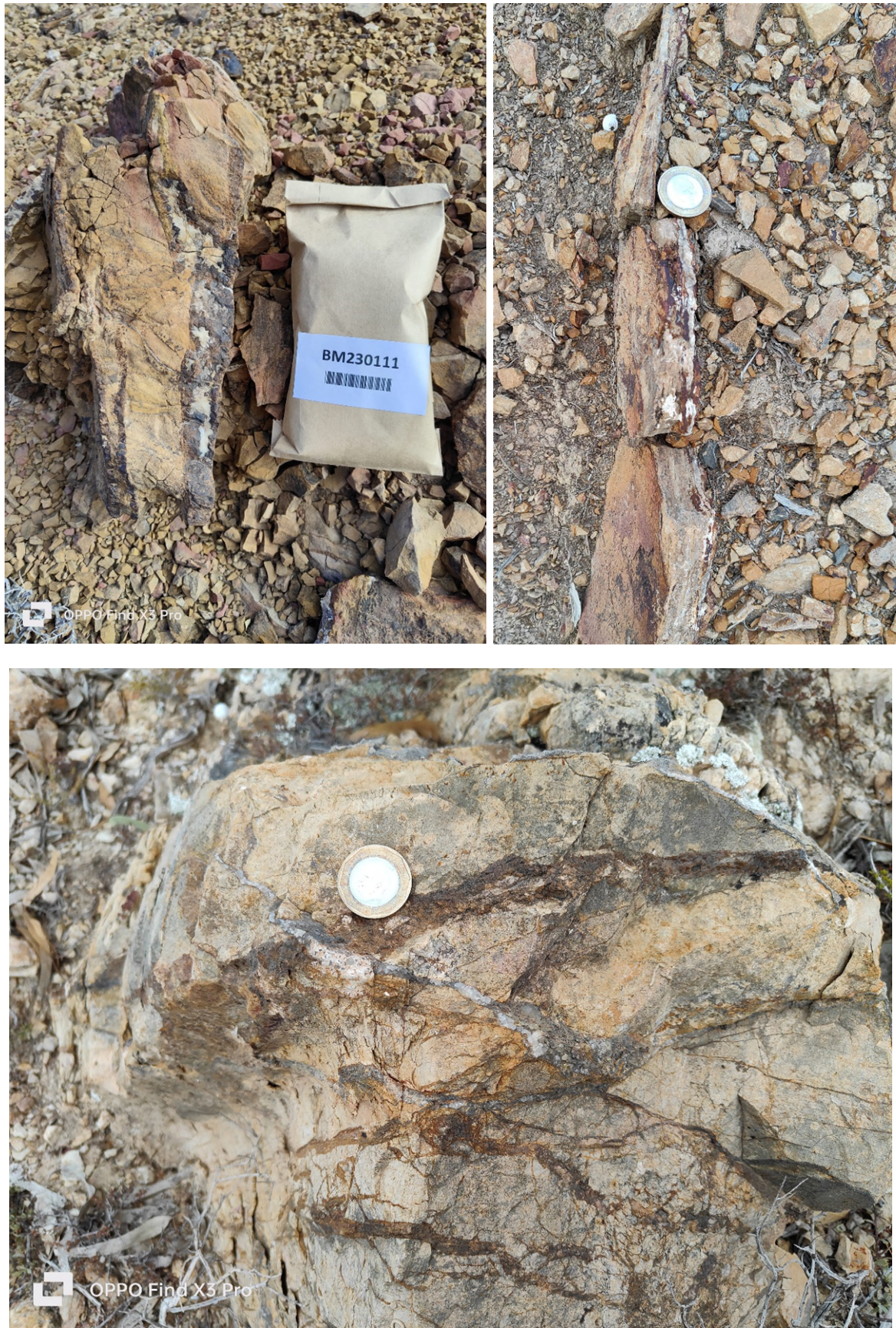
Figure 6. Typical quartz iron veins found in the stockworks
