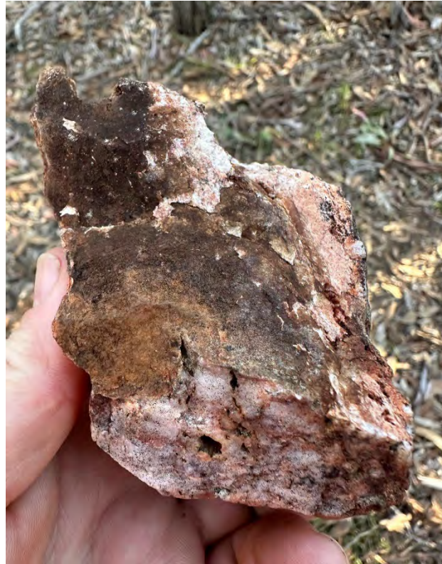
Figure 3 – Silver-Base metal mineralisation within ferruginous siltstone with quartz yielding 86 g/t Ag & >1% Ba from sample 3000782
