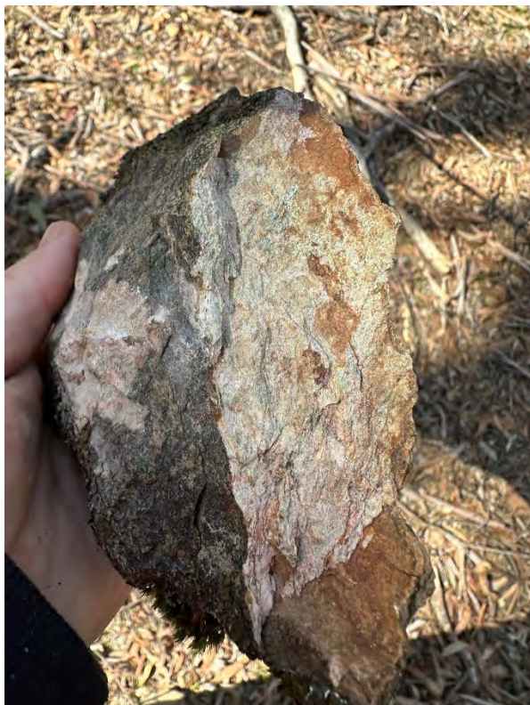
Figure 2 – Silver-Base metal mineralisation within ferruginous baritic sandstone yielding 99 g/t Ag, 0.22% Cu-Pb-Zn & 0.66% Ba from sample 3000768
