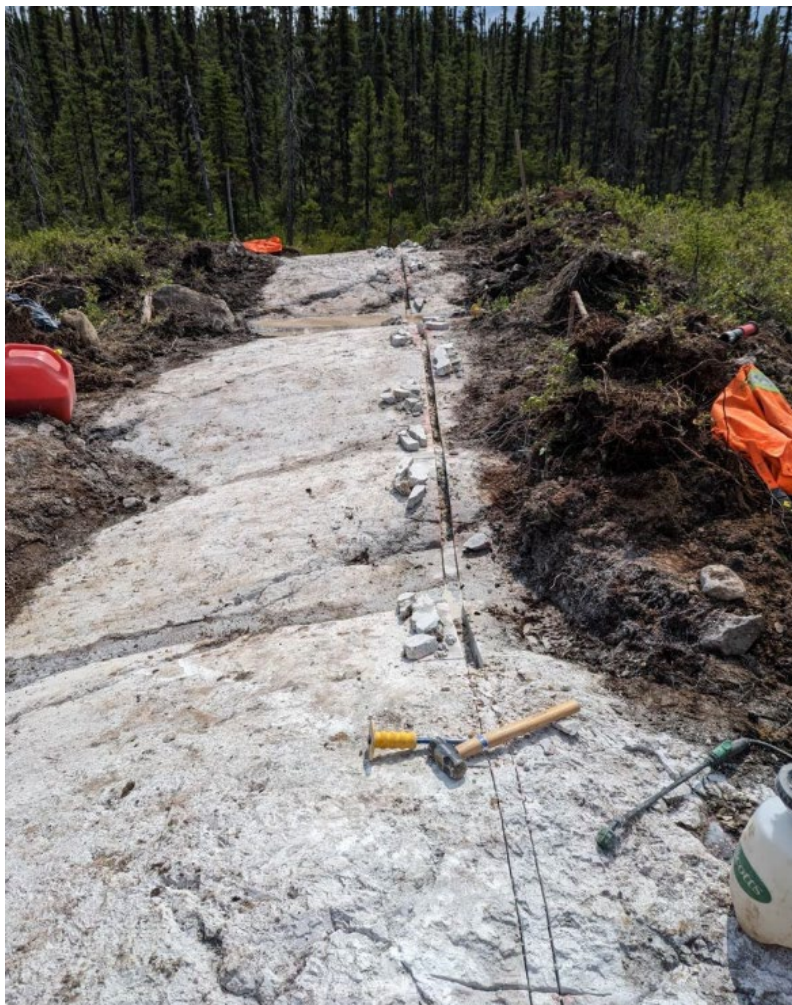
Figure 2: A substantial pegmatite outcrop at Ruby Hill West following removal of the layer of moss and vegetation. Drilling in the vicinity of this outcrop intersected 26.4m at 1.01% Li 2 O from 7.4m (see announcement dated 1 August 2022). NB this outcrop was discovered after the maiden drill program due to it being under shallow cover and covered in snow.
