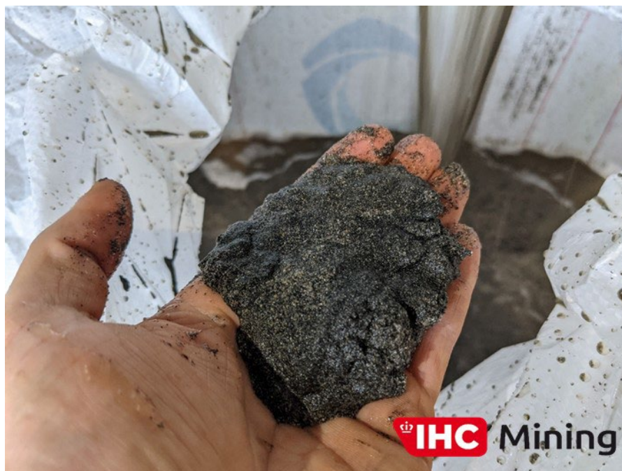
Plate 5 – Washed sand ready for industrial sand and magnetite-heavy mineral recovery (+2mm -45µm)
