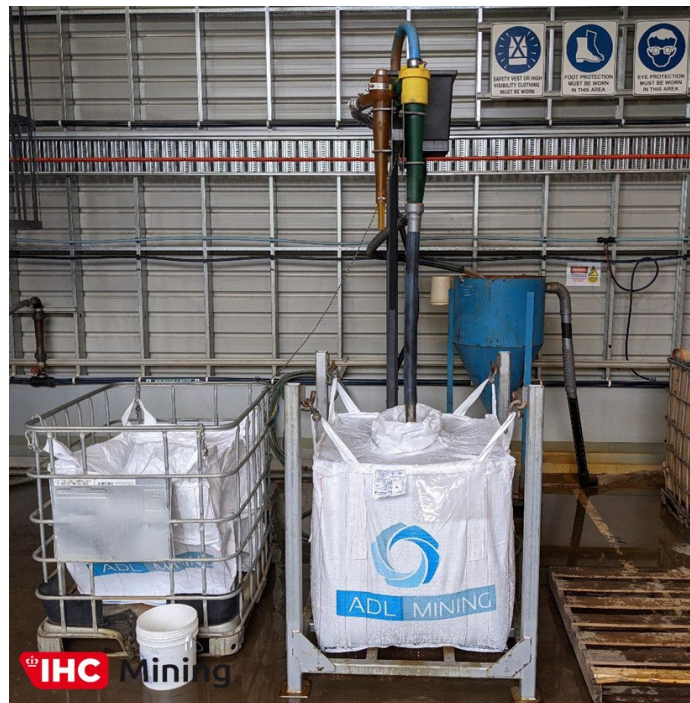
Plate 4 – Slimes removal (material <45µm)
