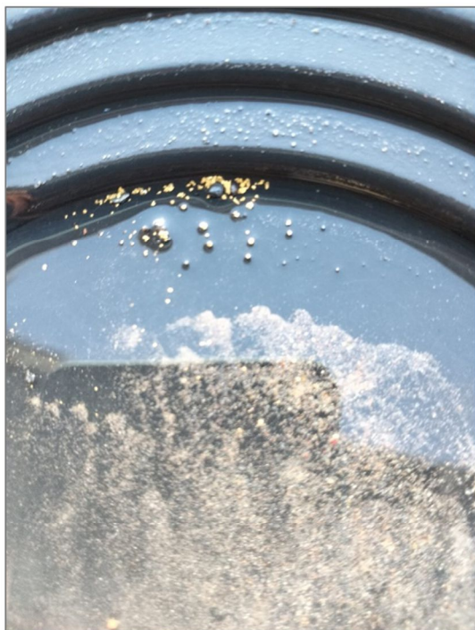
Figure 6. Single pan-concentrate containing 40+ visible gold grains, panned in the Camp-oven Ck area (see Table 2 for coordinate location).
