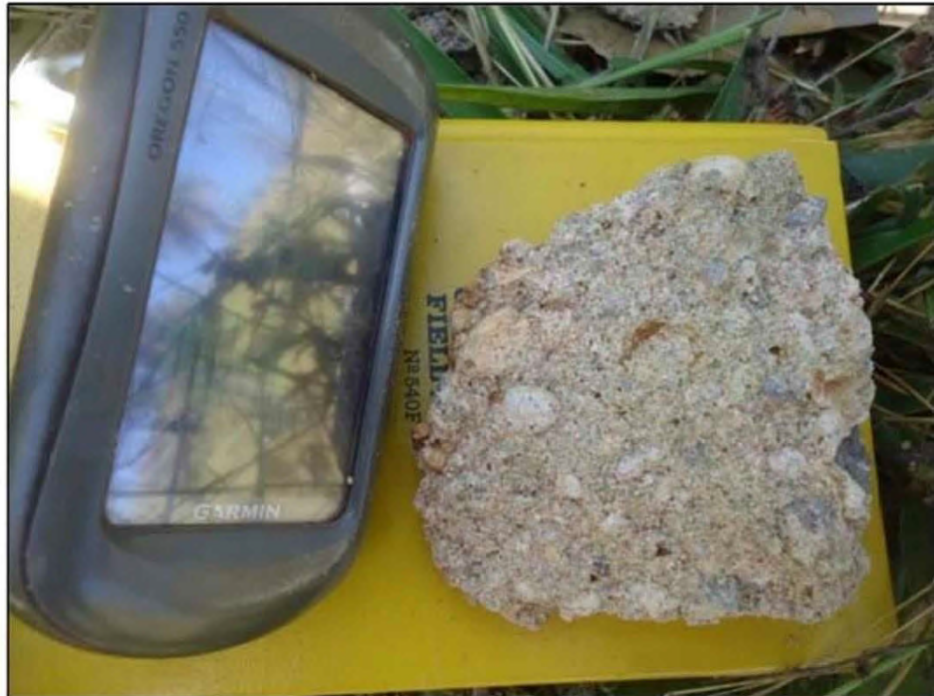
Figure 7-4 – Conglomerate hand sample from the Capacete Formation
