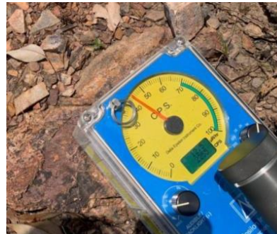
Elevated radioactivity from scintillometer (2,255cps)
