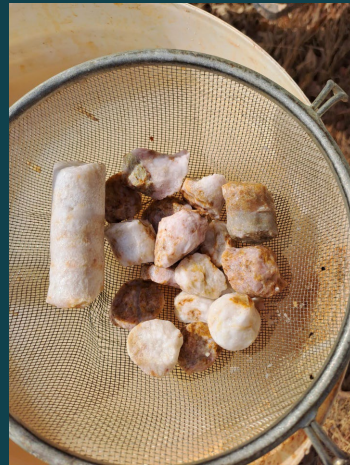
Quartz veining consistent with known mineralisation styles from the Northern and Central Targets on the Alice River Project, recovered from Aircore drillhole ARAC-107 1
