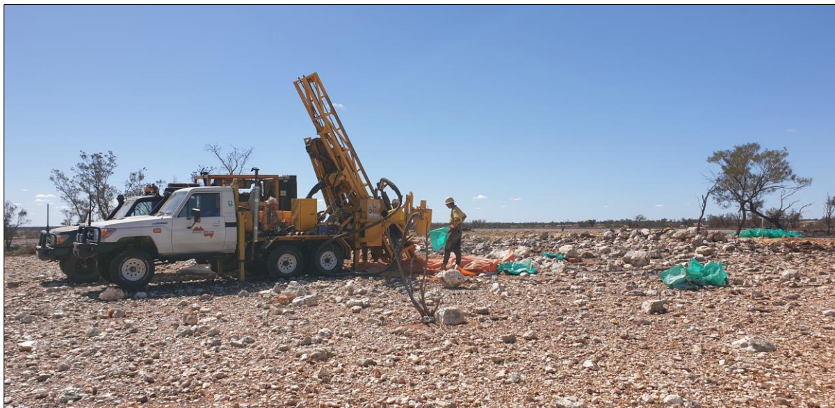
Photo 1. Aircore drill rig at the Bellagio Gold Prospect, with the main quartz vein outcrop shown to the right of the drill rig. Photo direction looking north east.
