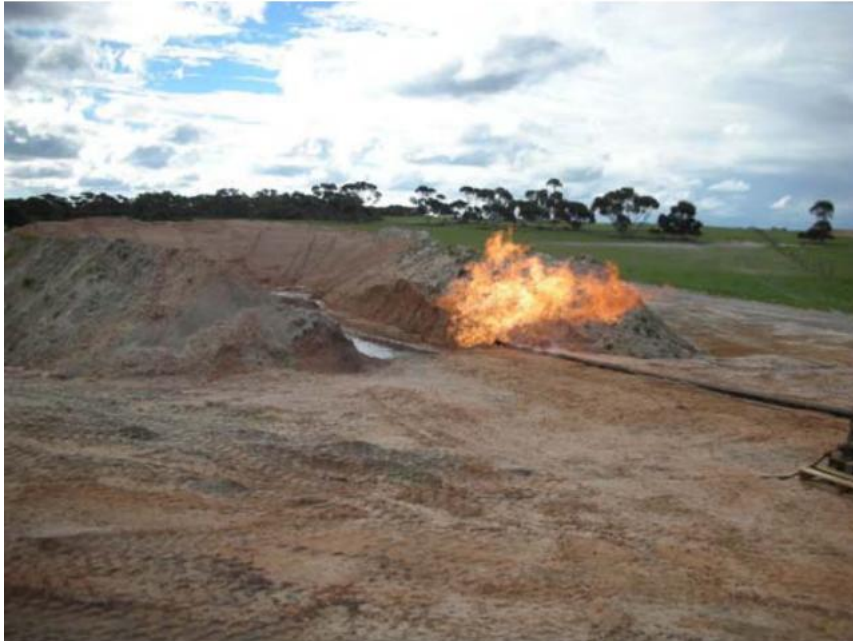
Figure 2: Warro 4 well test flare showing natural gas being flown at surface (Source: Warro-4 end of well report appraisal well testing).
