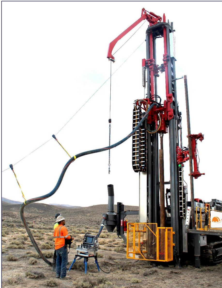
Figure 1 - Alford's Foremost Apex 65 RC Rig in operation (not Maverick Springs).
