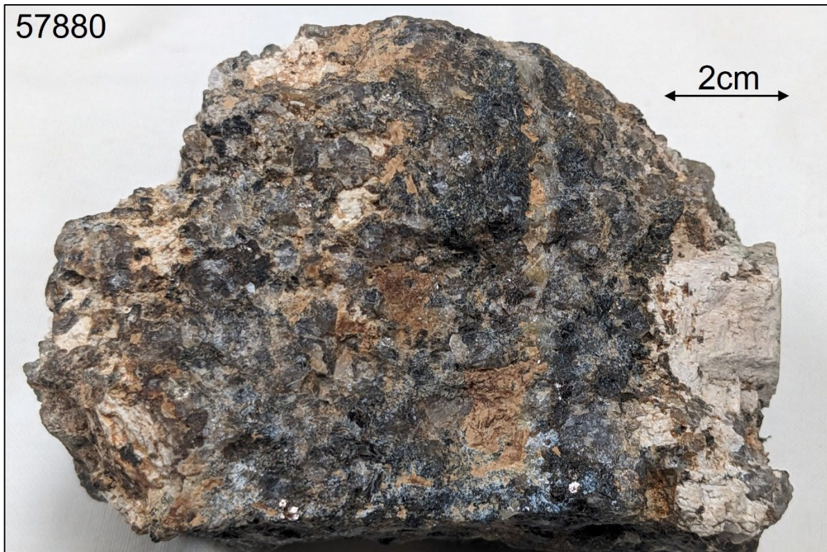
Figure 3: Photograph of rock specimen from sample 57880: cassiterite mineralised quartz-mica-topaz greisen with internal quartz vein (0.86% Sn and 0.16% \text{Li}_2\text{O} ).
