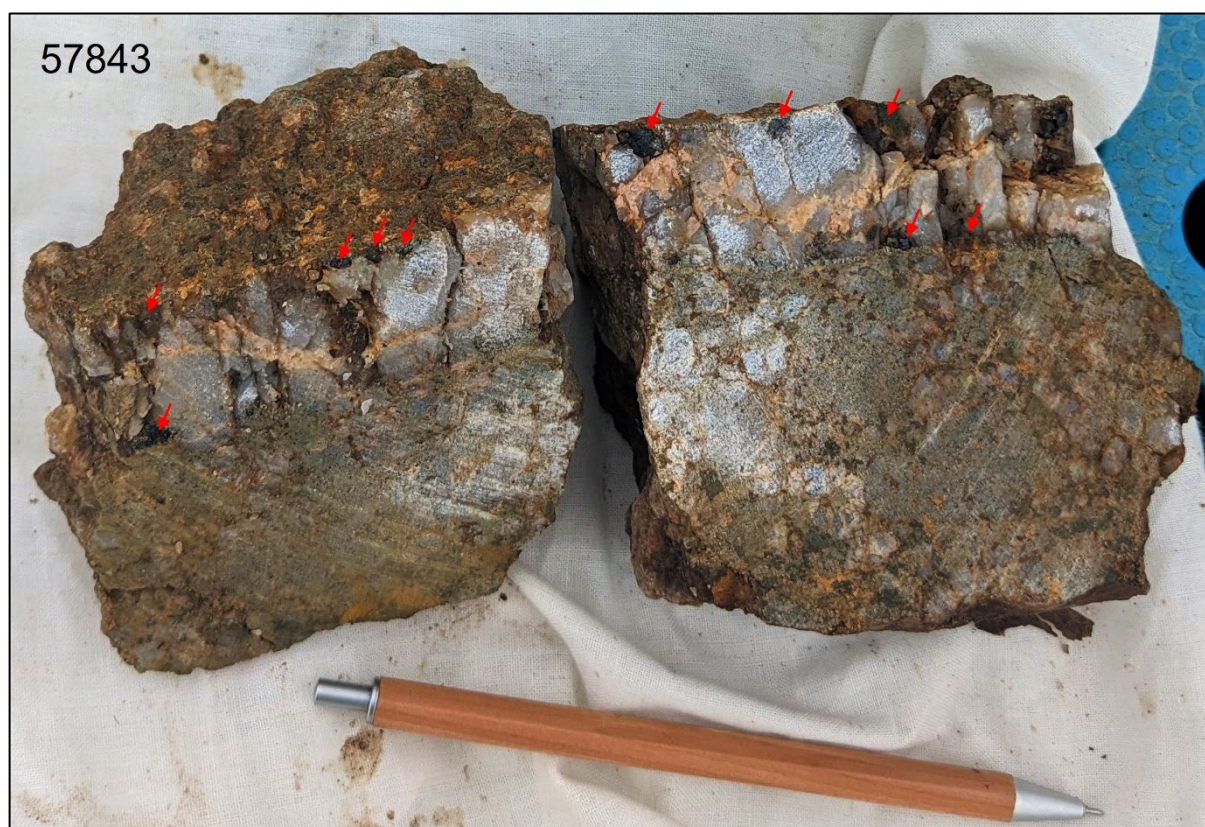
Figure 2: Photograph of cut rock specimen from sample 57843: cassiterite mineralised quartz vein in greisen altered granite (2.0% Sn and 0.03% \text{Li}_2\text{O} ). Red arrows indicate coarse cassiterite crystals (dark coloured crystals).
