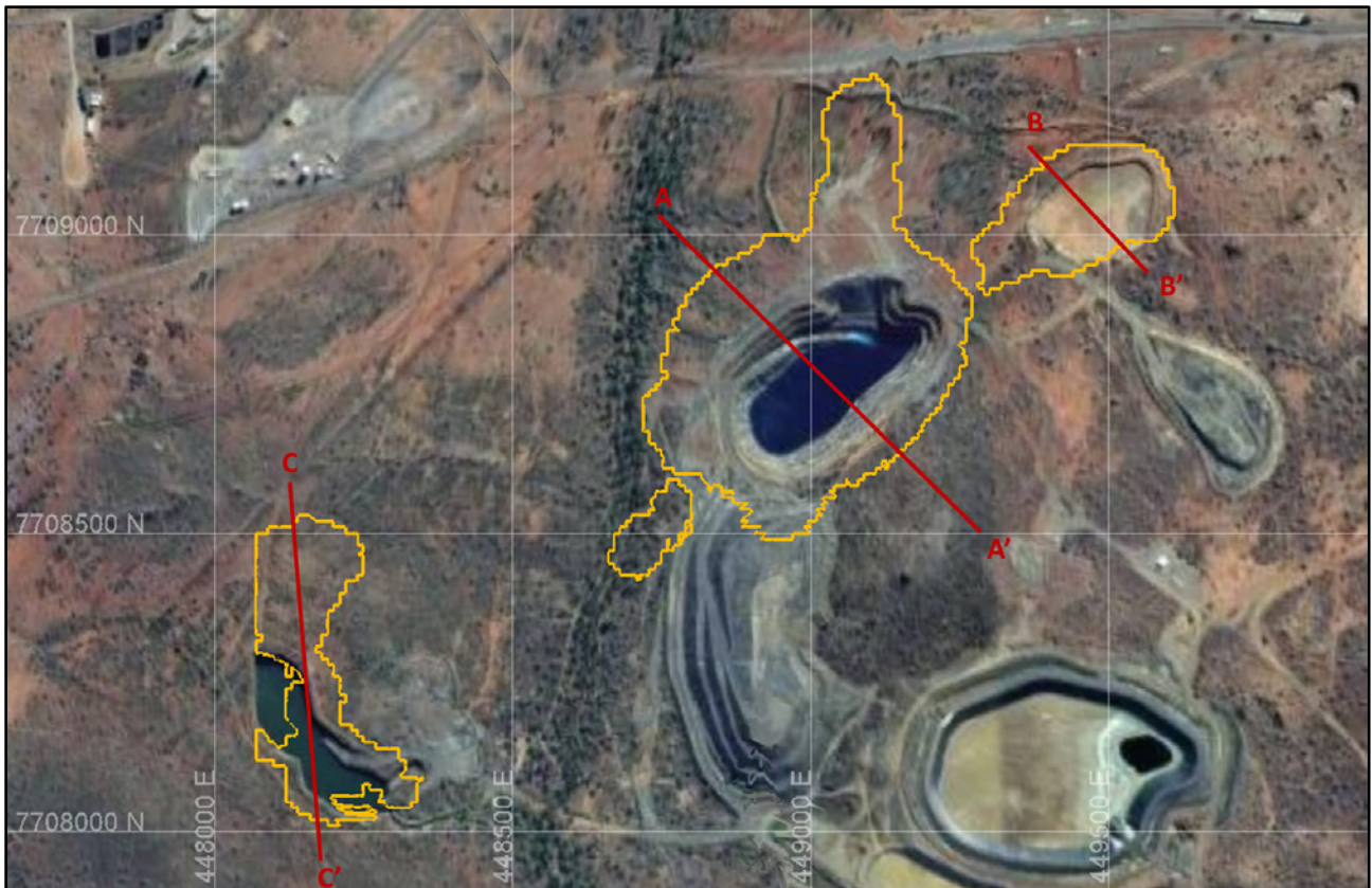
Figure 2: JORC 2012 Reserve Pit Shells for the Great Australia Mine (source MEC Mining)
