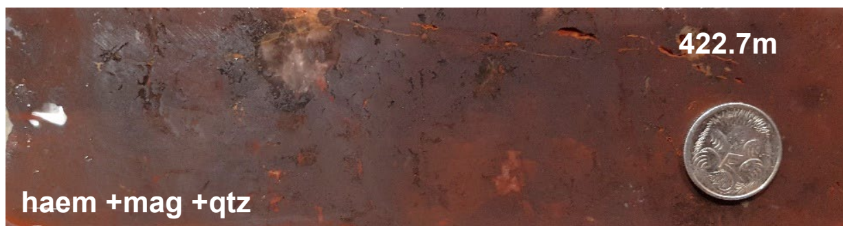
Figure 4 – Close up of ABNE 2 drill core at 422.7 metres down hole depth. Core has been replaced by massive hematite+magnetite+minor quartz alteration.
