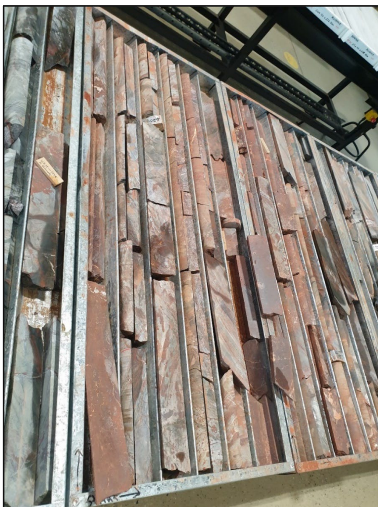
Figure 3 – Zone of strong hematite IOCG style alteration (rust red colouration) in hole ABNE 2 (interval 417.9m – 426 m down hole, not true width).
