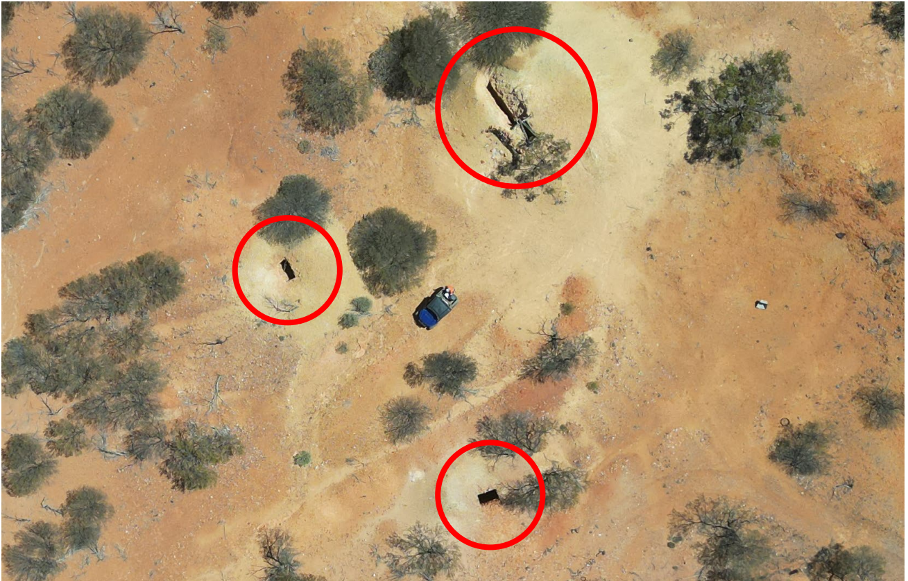
Figure 7: Drone image of Shaft 2 location showing three shaft collars and stope at the top of the frame.
