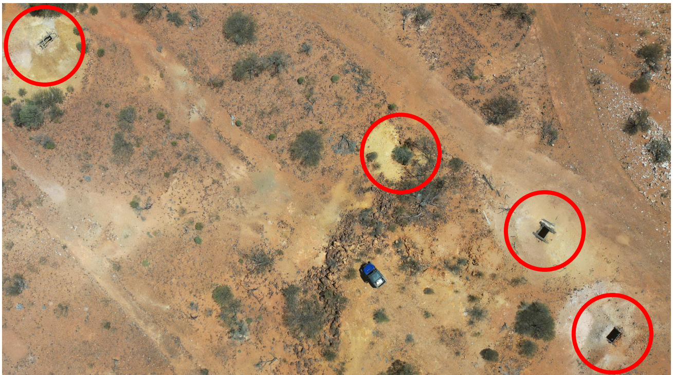
Figure 6: Drone image of Shaft 1 location showing four shaft collars. Historical diamond drilling at Shaft 1 intersected significant gold in the north-northeast splay orientation, including 8m @ 21.99g/t Au (BN003).
