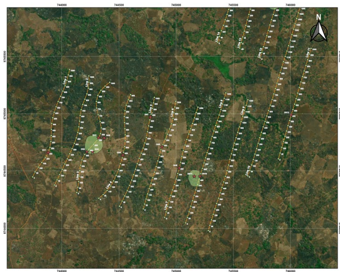
Figure 2: Planned RC Drill holes along the Southern Corridor of the Liparamba Nickel Project
