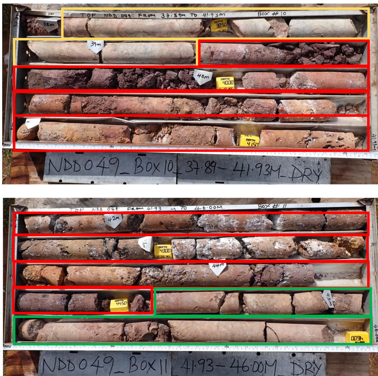
Figure4. Photos of core from NDD049 (39m to 46m) showing a thick intersection of logged weathered fluorite from 39.3m to 44.5m.
