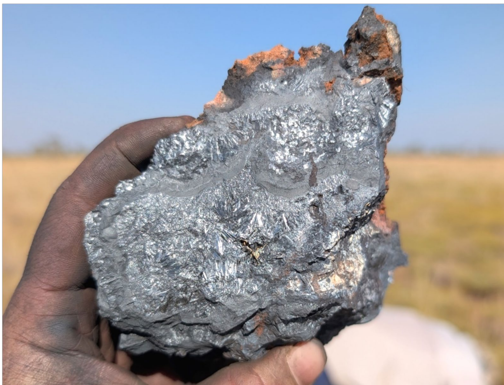
Figure 1. High-grade manganese rock chip sample example with 56.7% Mn (sample ID OS0063065) exhibiting apparent spongiostromate textures (finer grained domal layering formed from microbial mats - Stromatolites) hydrothermally replaced by high-grade manganese oxides along with other carbonates (white) that have not been subject to replacement.
