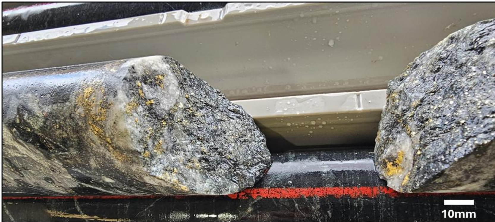
Hesperus visible gold intercept (0.5m intercept grading at 8,590g/t in GXDD0312)
