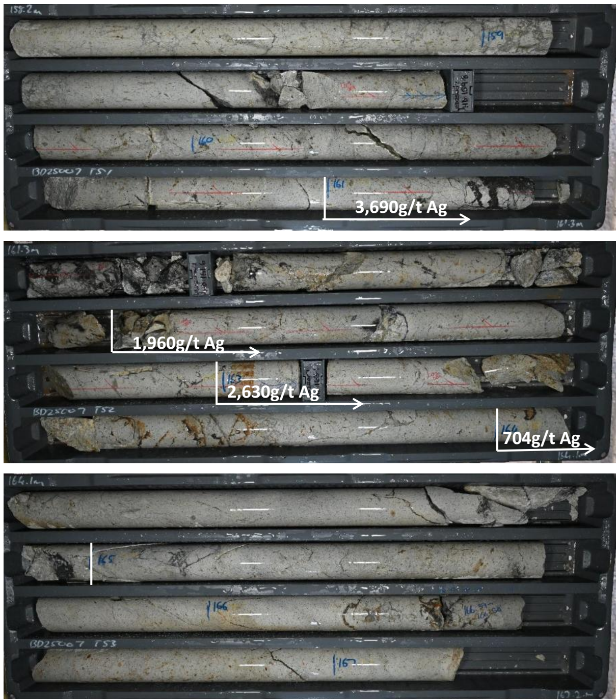
Figure 2: Core from significantly silver mineralised intercept from 161m to 165m in BD25007.
