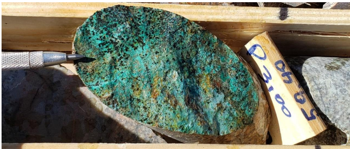
Figure 2. Drillhole PNSI22-002 at 59.40m: Equigranular granodiorite. Qz-Bt-Mt veins are altered with Fe and Cu oxidised minerals. This copper mineralisation at 59.4m is within the drill core sample PNSI22-2123 from 58 to 60m downhole depth, which contained 0.233% Cu. Refer to ASX announcement dated 11 October 2022.
