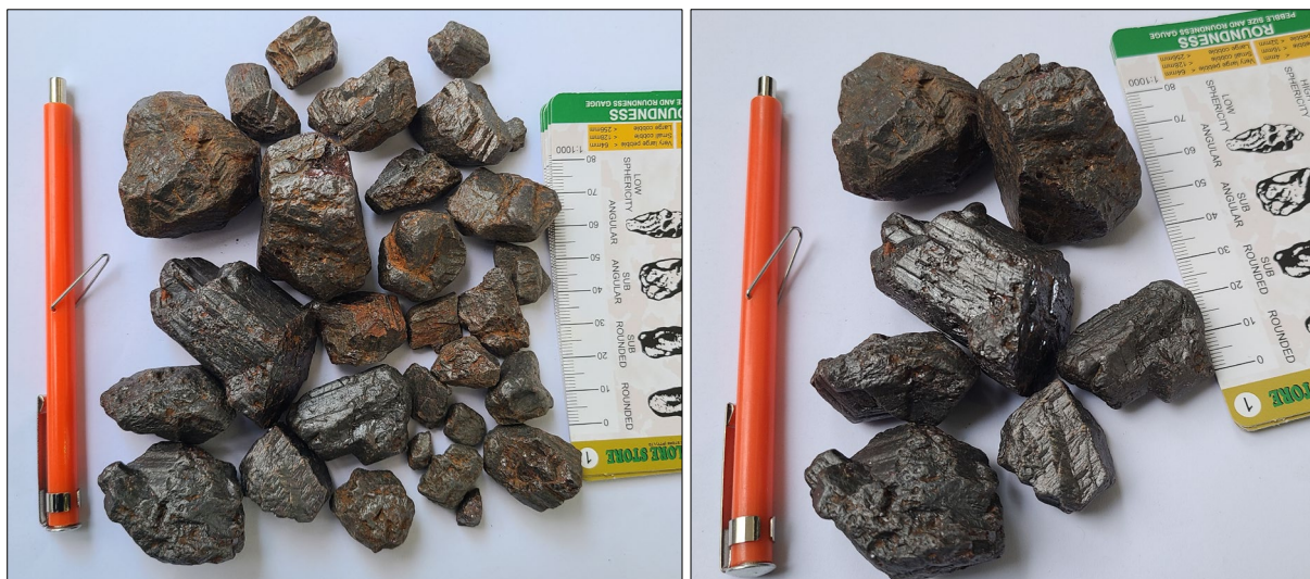
Figure 5: Widespread occurrence of eluvial coarse rutile exhibiting a massive texture, sub-metallic lustre, and black coloration with secondary Fe-oxides on some nuggets and subrounded crystals, suggesting limited lateral transport. It was recovered from residual regolith composed primarily of fine-grained, iron-rich soil and clay horizon in the area around soil sample KOMST0019 (UTM32N 800978, 416554) within the Kombo license.
