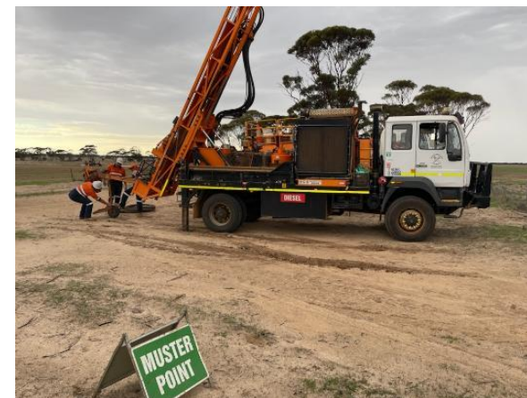
Salmon Gums Aircore Drilling Rig – May 2025
