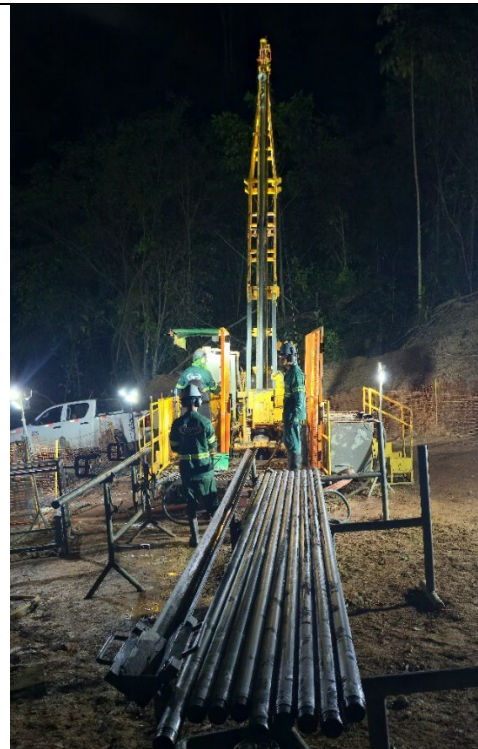
Figure 4: Top and Right - Diamond drill rig at VG1. Rig set up to drill VGADD0001 obliquely Mineralised Envelope to test interpreted cross-cutting structures. HQ core; Oct 2025; VG1 pad A. Operational photograph only.
