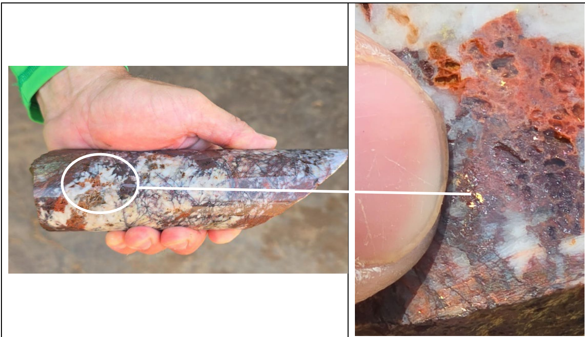
Figure 3: VGADD0002, 121.30–121.50 m (NQ core). Quartz-vein interval at the contact with the Interpreted Mineralisation Envelope showing localised visible gold (marked). Image unedited; colours not enhanced; thumb nail for scale. Visual observations are qualitative only; no sampling has yet been undertaken; assays are not yet available. Downhole lengths are apparent; true widths unknown.
