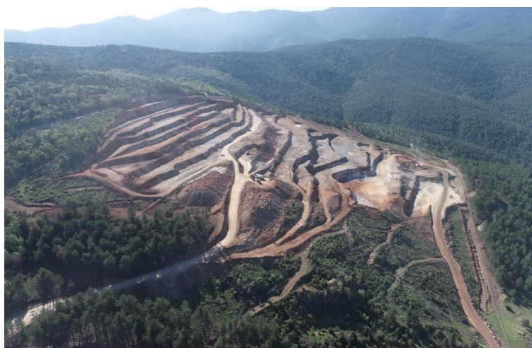
Figure 4: Tavşan Main open pit, showing the current status of open-pit development. Due to the shallow-dipping nature of the mineralisation, the stripping ratio has not exceeded 2:1 to date. Photograph taken in mid-May 2025.
