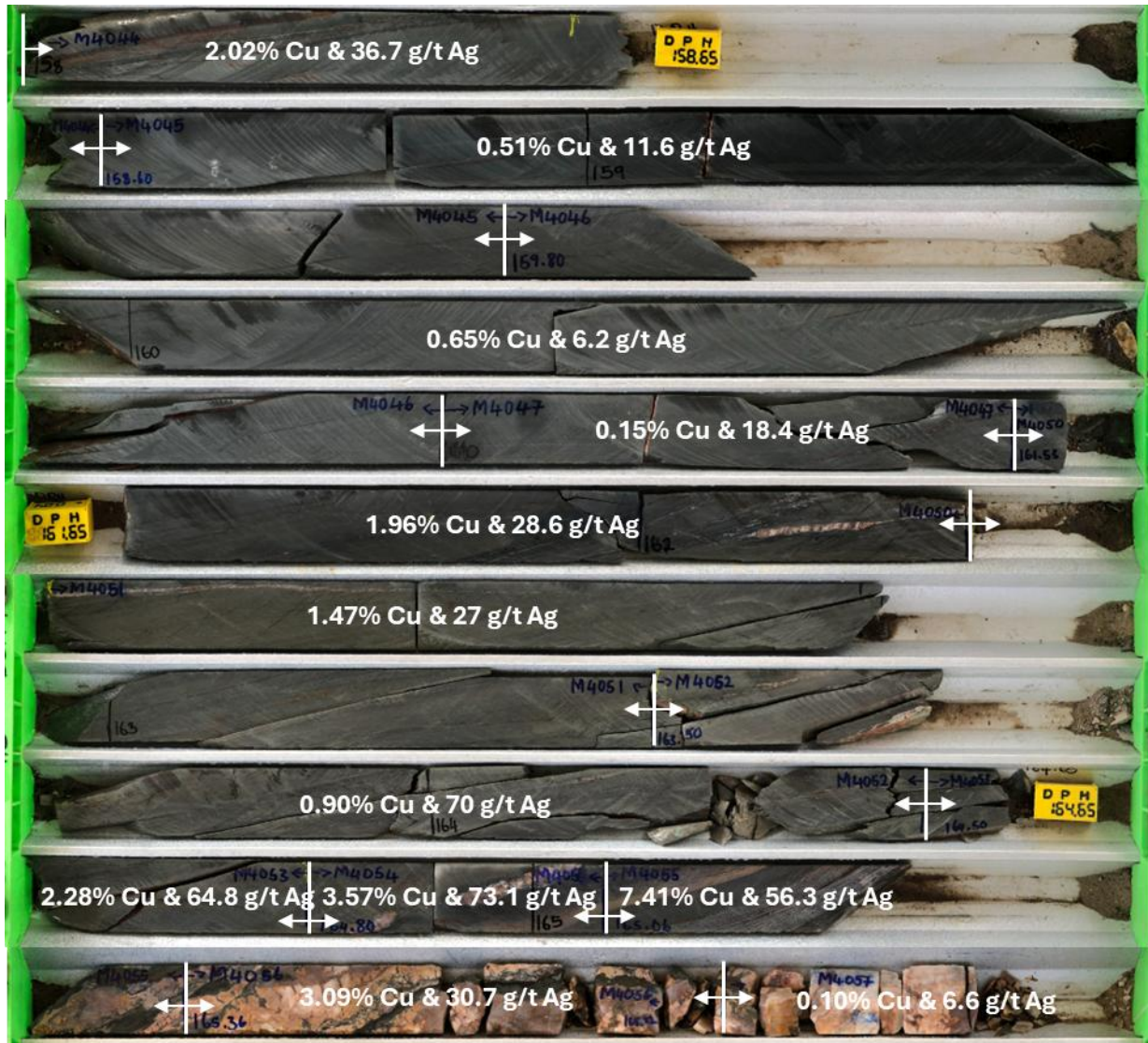
Figure 2. Drill core photos (HQ3 core) from NCP55 with sample results overlain. Note the increase in mineralisation towards the redox contact at the base of the figure with significant copper – silver assay values. See ASX Announcement 3 February 2025 for full JORC Tables related to the drill results from this hole.
