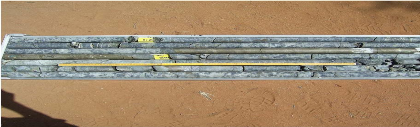
Maibele North: Ni + Cu in massive sulphide core
