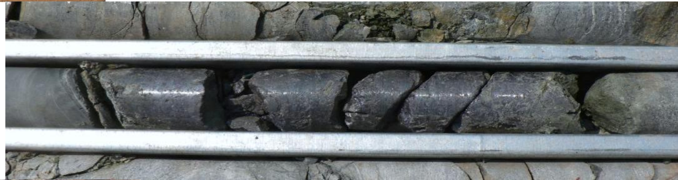
Airstrip: Cu + Ag in Bornite seen in diamond core
