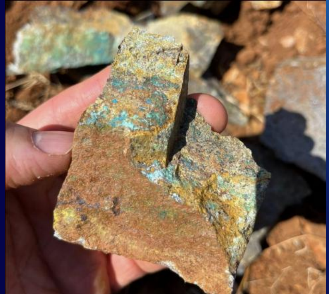
Above: Malachite mineralisation in trench sampling at Dibete (ASX release 20 September 2023)
