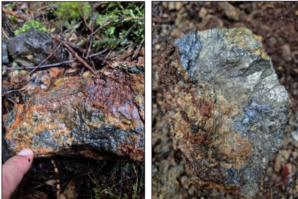
Figure 1: (Left) Sample ER25001 with sphalerite-galena-siderite vein, and (Right) ER25002 massive jamesonite and pyrite vein sampling 3,550g/t Ag and 14.7% Sb.
