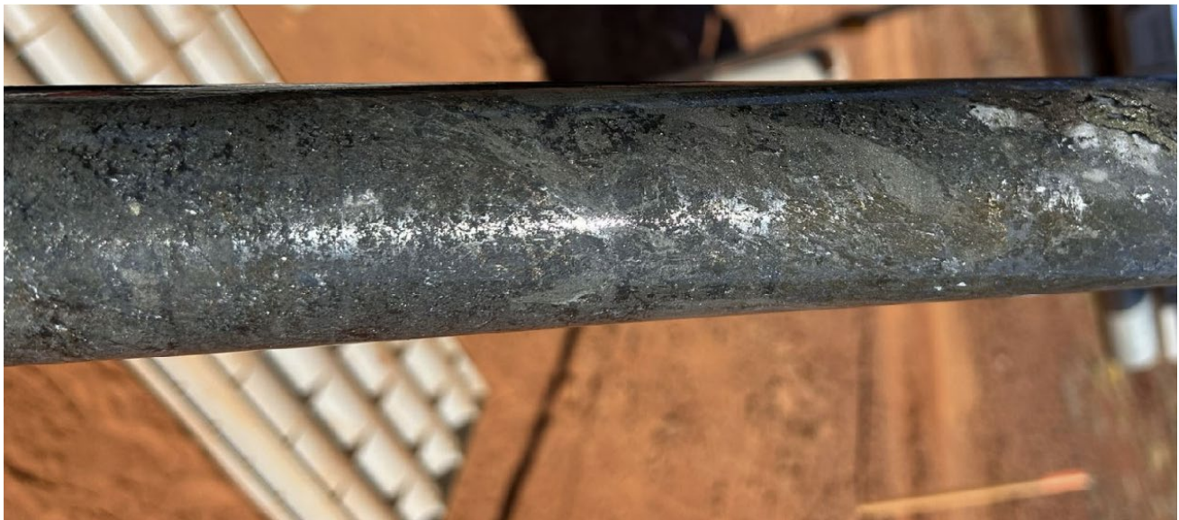
Figure 4: Core from drillhole EHDD25001 (~240m depth) showing semi-massive sulphide mineralisation (pyrite-pyrrhotite-boulangerite (Pb5Sb4S11) within a zone of quartz-sulphide stockwork veining. Sulphides in this interval constitute ~50% of the rock shown. Assays are pending for this interval.
