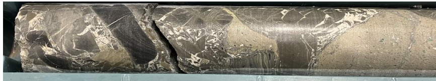
SDDSC079, 548 m; Complex dyke-sediment interaction, with dyke fragments (beige), altered and unaltered sediment fragments, with partial quartz vein matrix.
