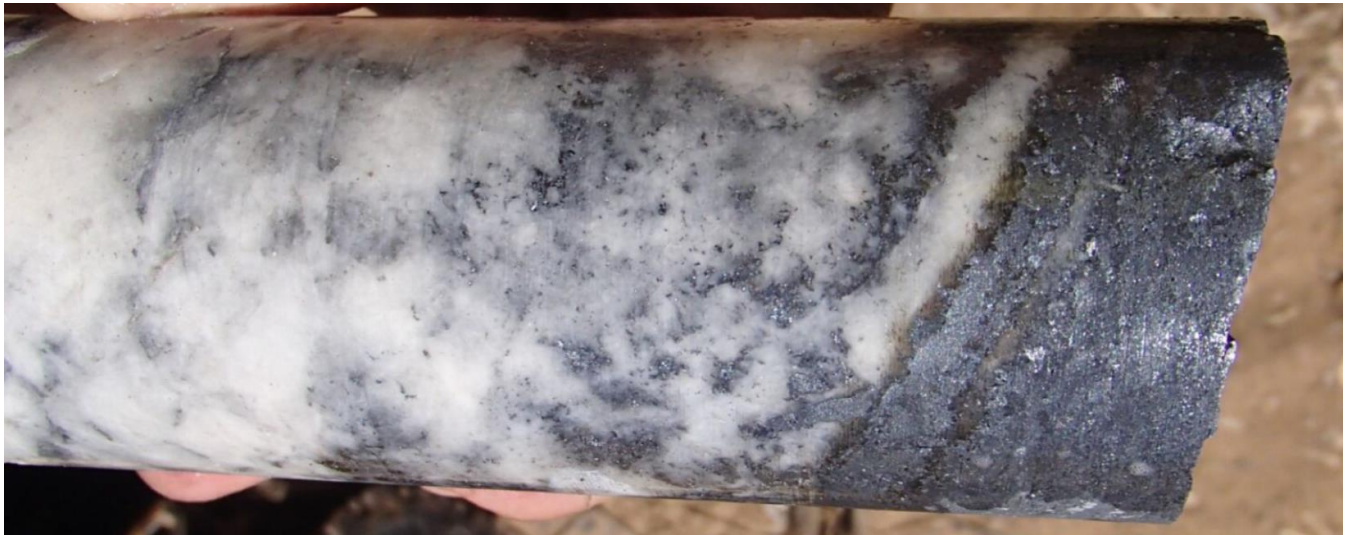
Figure 5: NQ drill core from 131.45m depth from CBADD003. Massive stibnite on the right of the core from 131.6m, with quartz and stibnite to the left. Detailed logging and sampling are underway, assays expected in November 2025.
