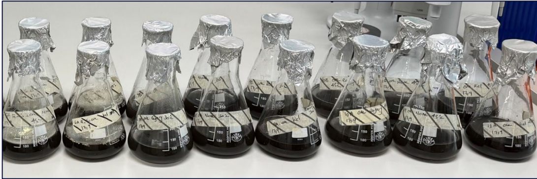
Photo 1: Bioleaching flasks with Brumby HEBS material mixed in various substrates and microbe content to identify the most effective conditions and temperature for leaching.
