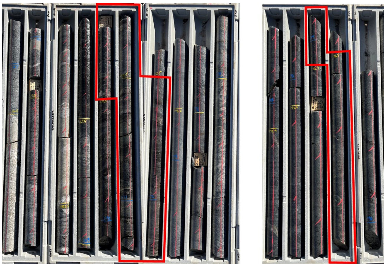
Figure 3. Sulphide rich zones in BDCDD2503 at 170.5m-172.5m downhole and 194.9m-195.9m downhole.
